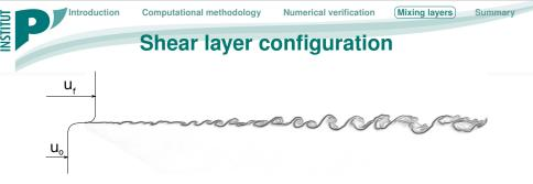
$\begin{array}{l} L_x \times L_y = 350 \delta^0_{\omega} \times 90 \delta^0_{\omega} \text{ with } N_x \times N_y = 2085 \times 455. \\ R_{\omega} = \bar{\rho} \Delta u \delta^0_{\omega} / \bar{\mu} = 640, M_c = \Delta u / (c_f + c_o) = 0.4. \end{array}$
