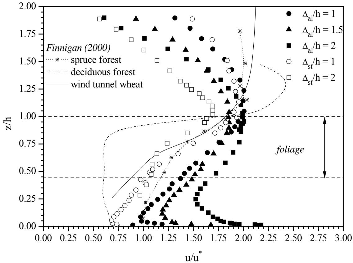
Root-mean square longitudinal velocity profiles
