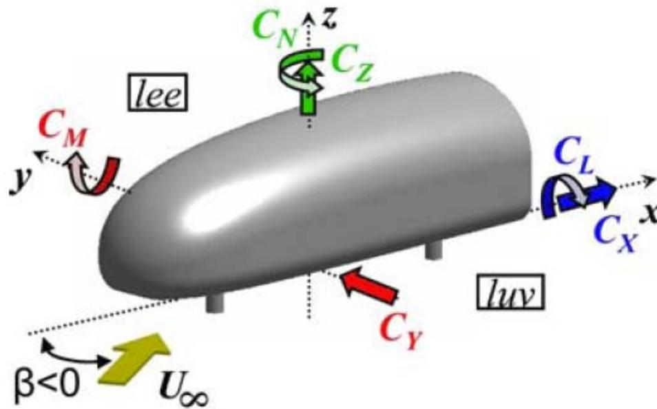
(b) Image of the three dimensional force tensor in the model fixed coordinate system
