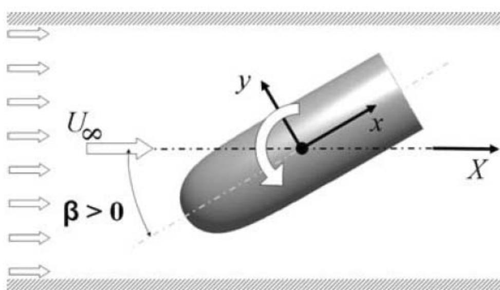
(a) Orientation of the model in the wind-tunnel set up
