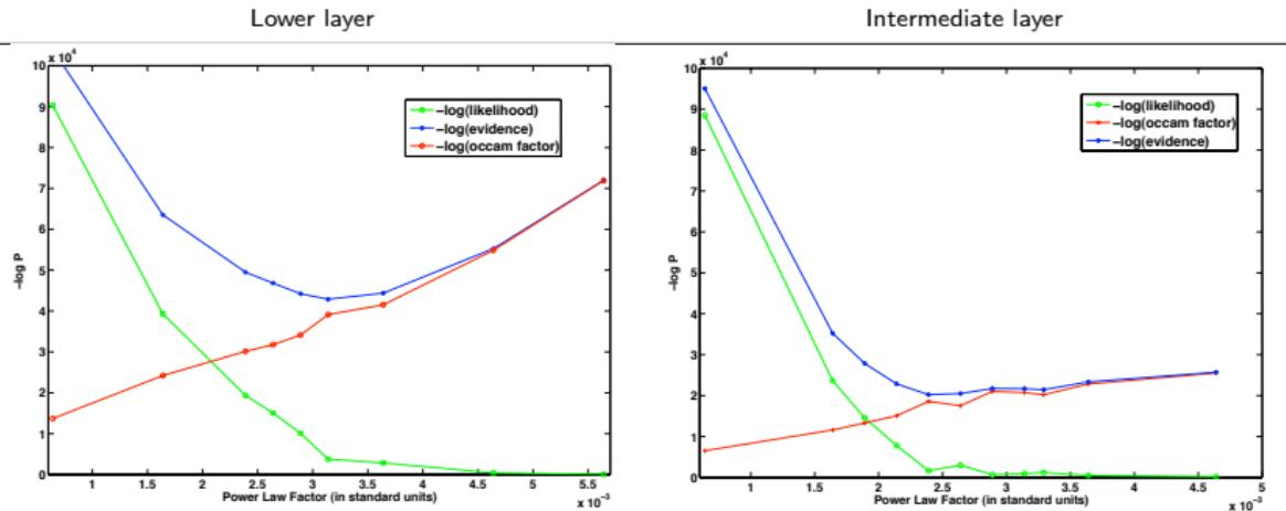
**Scaling law model evidence.** Behavior of *data term*, minus the log evidence and of minus the log of occam factor w.r.t factor  $\beta$
