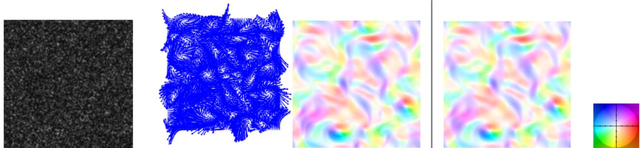
Left : particle image obtained by DNS of 2D Navier-Stokes equations & true velocity field.
