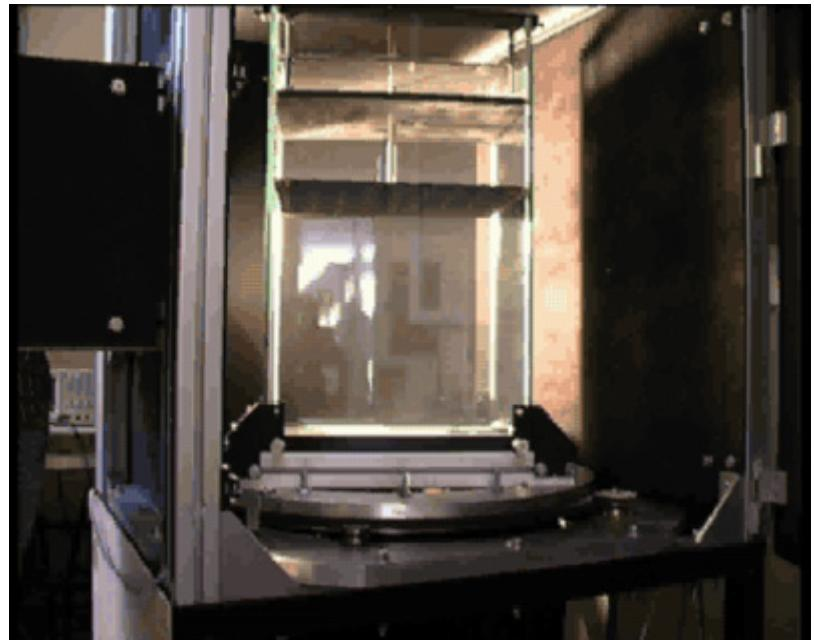
Grid velocity:  $V_g = 0.65 \text{ m/s}$  ( $Re_g = 2.5 \cdot 10^4$ )
