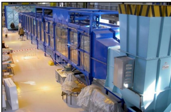
Atmospheric boundary-layer wind tunnel at LHEEA lab.
