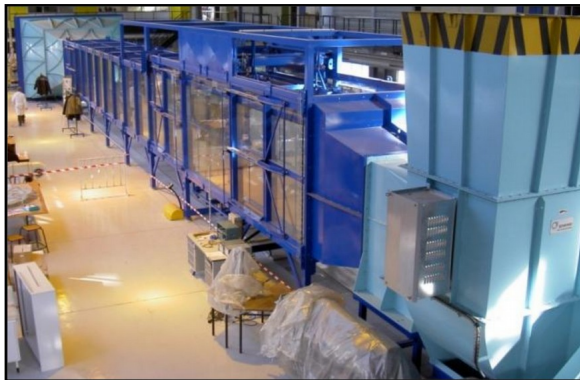
Atmospheric boundary-layer wind tunnel at LHEEA lab.
